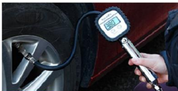
2nd Step Reading the Pressure
