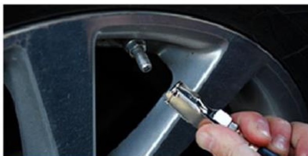
1st Step Connecting Tyre Valve
